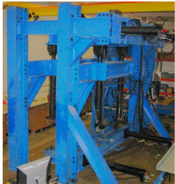
(b) MDOF testing rig in the JHU Structures Lab
