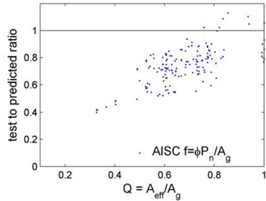
**Figure 12 Test-to-predicted strength for cold-formed steel columns failing in local buckling if the current AISC Q-factor method was used in cold-formed steel design, AISC (2001) Q-factor method, NAS (2001) for effective width calculation with  $f = \phi_c P_n / A_g$  to determine Q, 156 cold-formed steel column tests from Schafer (2002) local buckling only.**
