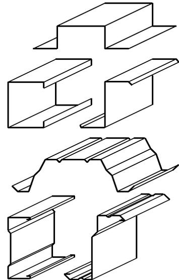
**Figure 3 (above) Typical cold-formed steel shapes created in the U.S. in the 1940’s and still used today (below) more optimized shapes**
