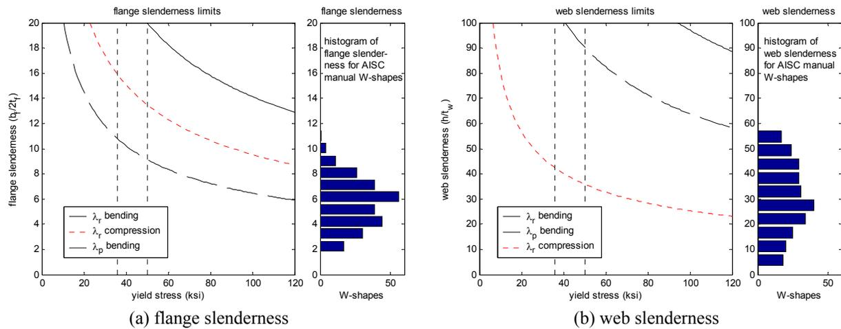
**Figure 5 Impact of yield stress on slenderness limits compared with current slenderness of W-shapes**
