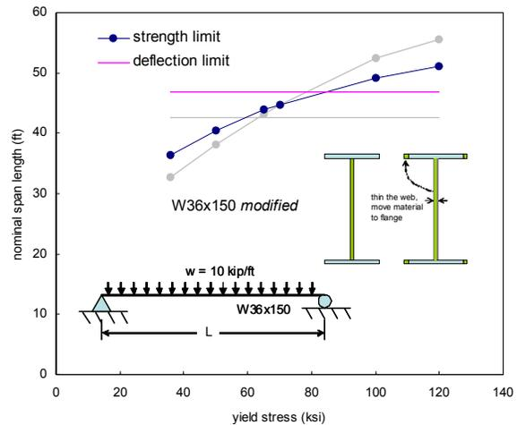
**Figure 7 Example of benefits of shape optimization for a conventional W-shape when using high strength steel, modified section has the same weight/foot and depth as original W36x150, material from the web is moved to the flange, but the section is noncompact essentially over all yield stress (a variation of DSM is used to approximate the strength shown.)**
