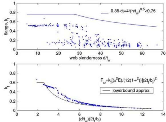
**Figure 11 Local plate buckling coefficients for all W-Shapes in the AISC (2001) manual in pure compression**, results based on elastic buckling finite strip analysis, for common W-Shapes used as columns the web is significantly more slender than the flange and reduces the flange  $k$  considerably.
