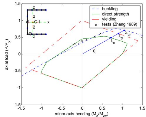
**Figure 10 DSM applied to a beam-column**
