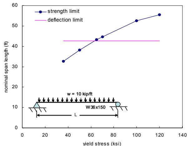
**Figure 6 Simplified example of the limits of increasing yield strength on conventional sections, span length as a function of yield stress for a fully laterally braced W36x150 under 10 kip/ft uniform load (nominal calculation: no safety or resistance factors)**
