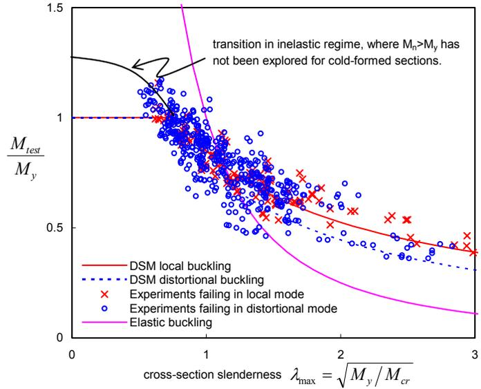
**Figure 4 DSM predictions compared with experimental data from 569 cold-formed steel laterally braced beams, note the elastic buckling curve shows regimes where elastic post-buckling is assumed in the prediction equations, also extension to structural steel will require closer examination of inelastic regime  $M_n \rightarrow M_p$**
