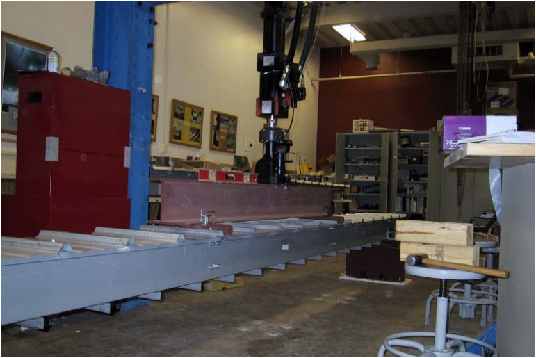
Figure 4 Phase 1 testing setup (top panel in the constant moment region will be removed and dist. buckling allowed to occur in Phase 2)
