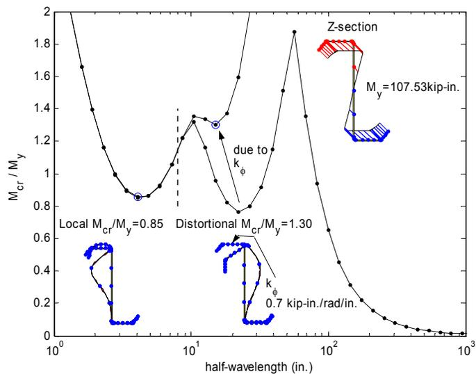
**Figure 7 Example of impact of adding rotational restraint to the flange
