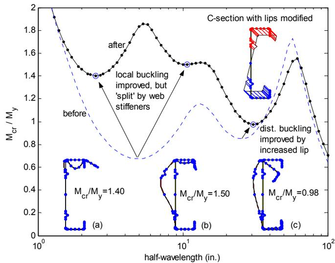
**Figure 6 Example of modified/optimized C-section
