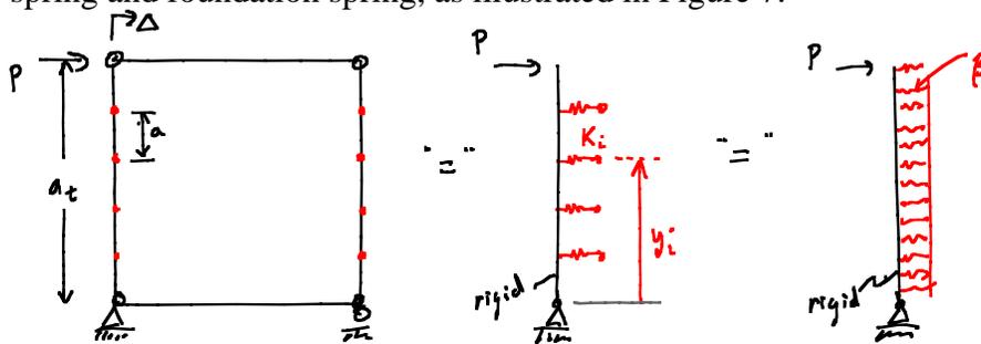
Figure 7 Lateral spring models for diaphragm test
