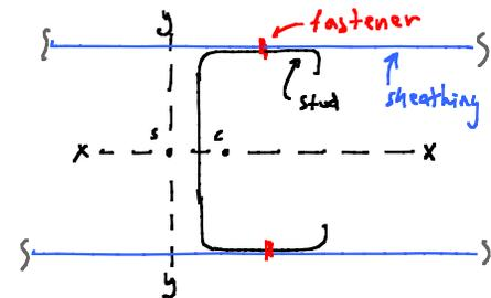
Figure 8 Stud and typical coordinates
