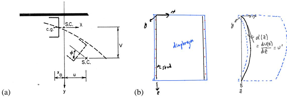
Figure 4 Coordinate system (a) Simaan and Peköz (1976) Fig 2 (b) additional notation
