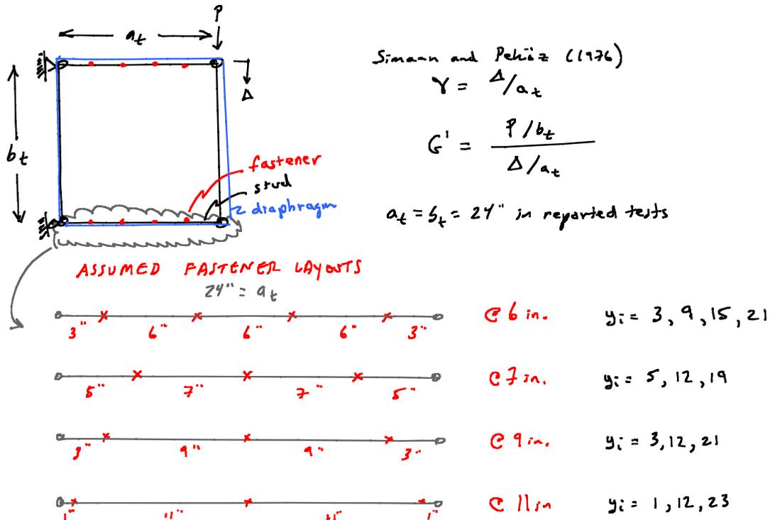
Figure 6 Details of diaphragm testing reported in Simaan and Peköz (1976)
