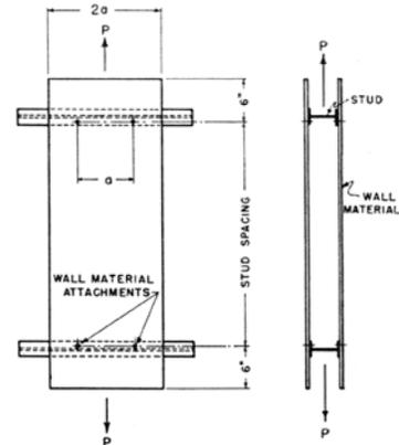
Wall Material Test Assembly
