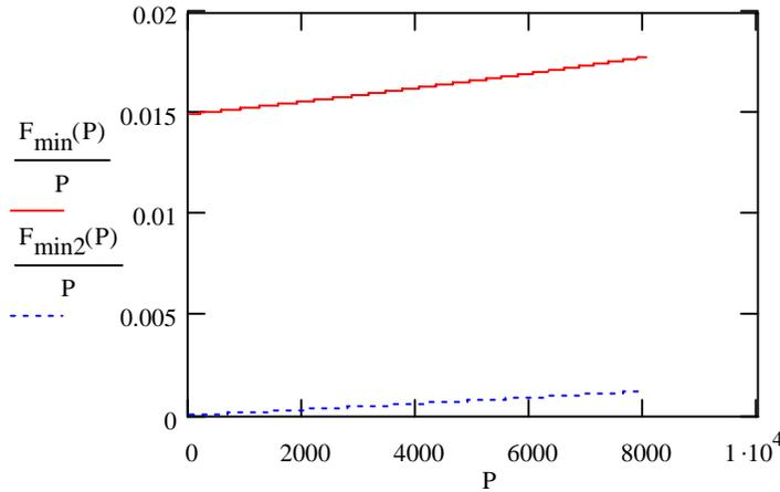
Figure 2 Required fastener forces for Example No. 11 of AISI (1962)
