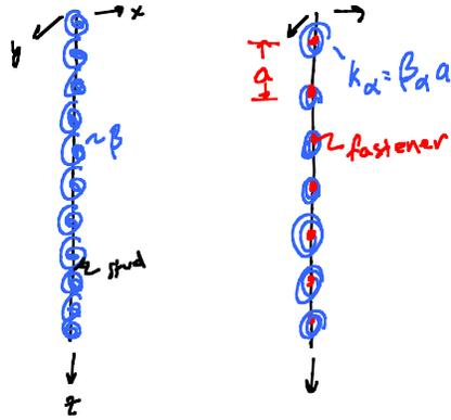
Figure 5 Rotational spring model equivalent to shear diaphragm model of Simaan and Peköz (1976)
