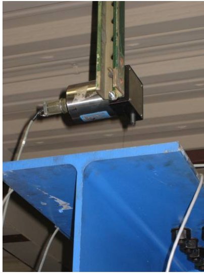
a) String Pot, checking actuator displacement
