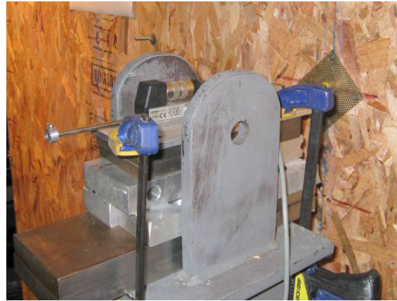
b) PT checking displacement out of the wall plane
