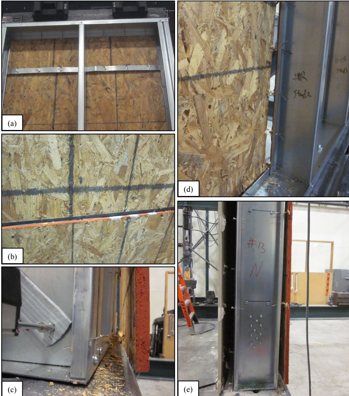
Figure 6: (a) Back of test 4, demonstrating fastener pull-through (PT) along the horizontal seam (b) front of test 2 depicting the resulting separation of sheathing from seam as a result of PT (c) separation of OSB from bottom wall track in test 13 (d) Fastener PT and tear-out (TO) against sheathing along field stud in test 11 (e) north chord stud in test 13, demonstrating fastener PT in the OSB and a combination of PT and bearing (B) in the gypsum.
