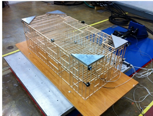
Figure 6. A 1/12 th -scale CFS-NEES building made of balsawood.
