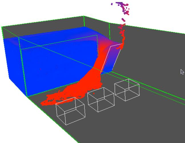
Fig. 5. Failing floodwall section, early stages. Note that the flow is alongside the levee and that there is an initial spray off the top of the falling wall.
