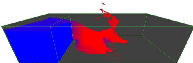
Fig. 4. Three dimensional dam break, with the flood flow striking three structures. At the depicted instant, the first structure closest to the jet center line, is completely overwashed and the jet is deflected into the air. Flow is occurring between that structure and the next. Run-up on the second structure is occurring.
