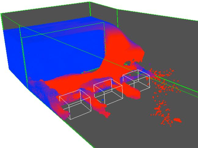
Fig. 6. Failing floodwall section. Flooding occurring between the homes. Note the run-up on the front of the homes.
