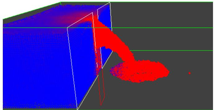
Fig. 8. Dropping floodwall section, showing the weir behavior of the flow from the levee.
