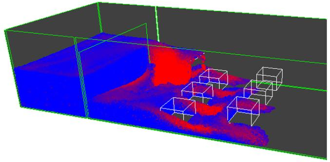
Fig. 7. Failing floodwall section, with six structures, which are located in a staggered pattern so that the flow can not go directly through the structures.
