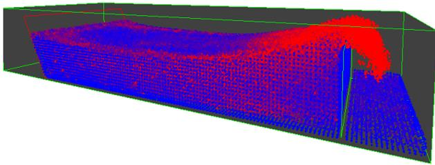
Fig. 3. A second wave overtopping the floodwall. The different trajectory of the overtopping jet is a result of the influence of reflected waves in the levee system.
