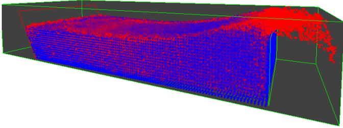
Fig. 2. Flood wall, at incipient overtopping by a large wave. The fluid is color coded to represent velocity, with the highest velocities occurring in the overtopping jet.
