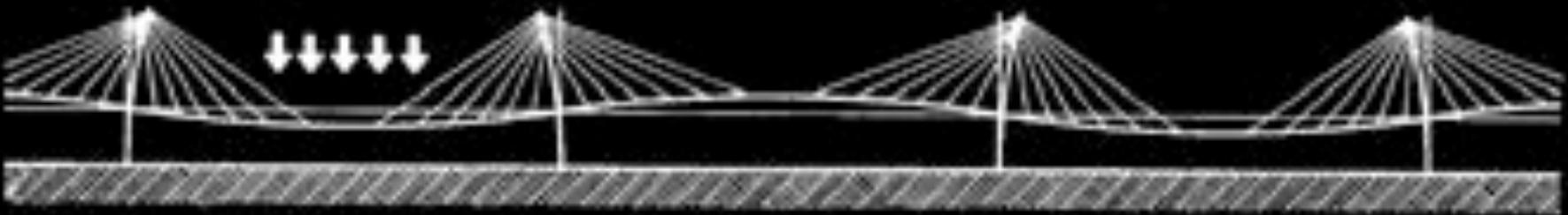
c. Loading an adjacent span
