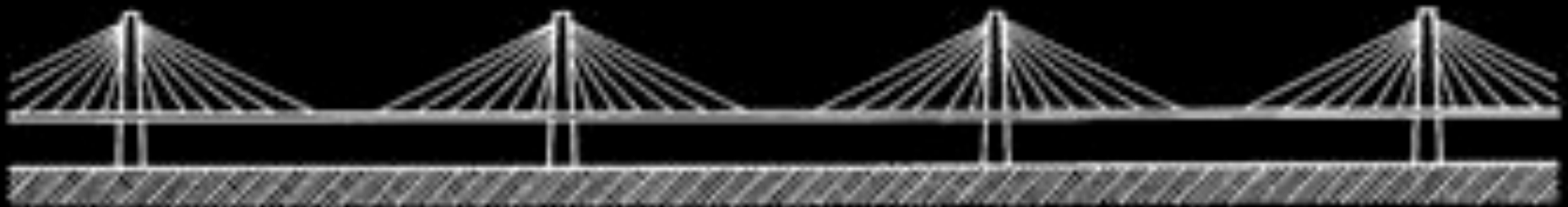
c. Rigid pylons and flexible deck, with a transmission of moments between pylons and piers.
