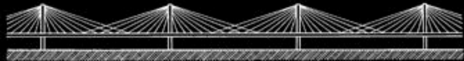
d. Cable-stays coming from both adjacent pylons to support the central part of each span.
