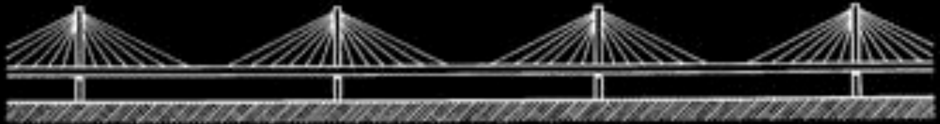
a. Rigid deck, with different possible types of connection between deck and piers.
