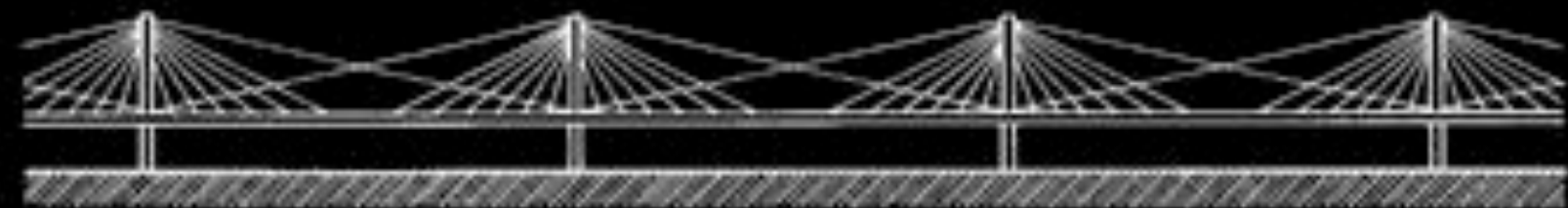
c. Long cables from a pylon head to an adjacent pylon at the deck level.
