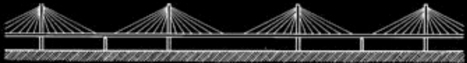
a. Intermediate support every second span.
