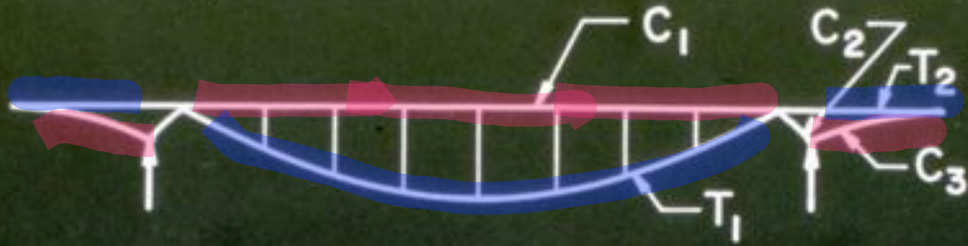
(a) CONSTANT FORCE TRUSS
