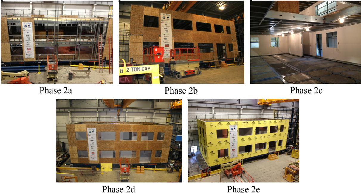
Figure 3: As-built sub-phases of Phase 2 testing. Note, in Phases 2c and 2d, additions are only made to the interior of the building.
