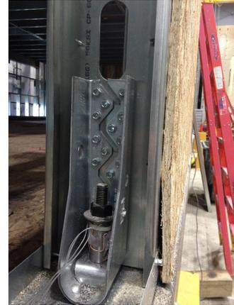
Figure 7: Left: Phase 1 building at peak drift, with plots of hold down forces. Clustered hold down forces (all red, for example), indicate Type 2 behavior. Right: photograph of load cell installed in shear wall hold down.
