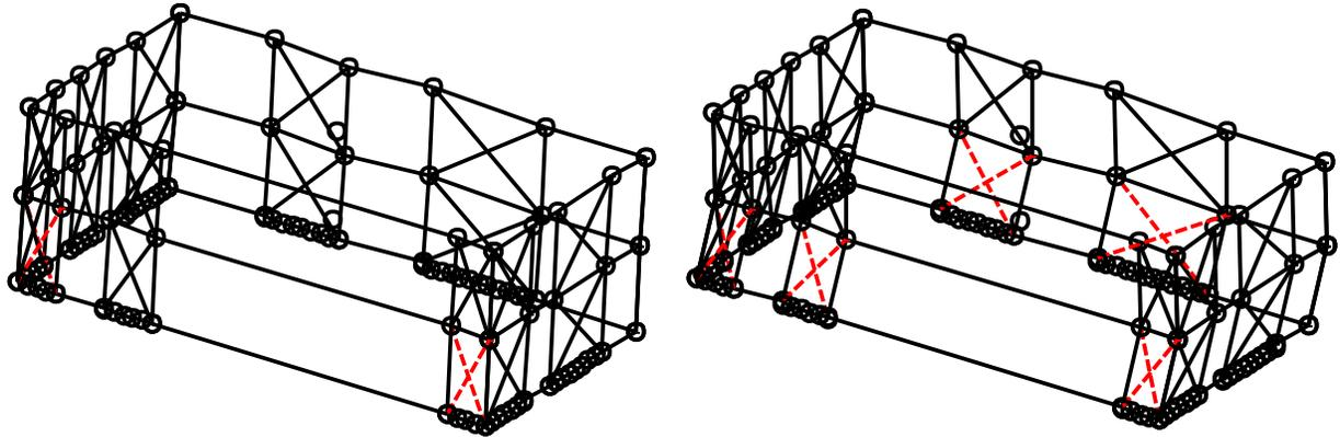
(a)  $t = 2.0$  sec. (b)  $t = 5.18$  sec. (max base shear in x direction)
