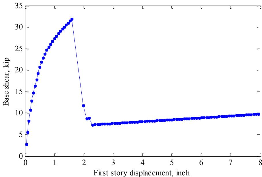
Figure 8: Pushover curve of 3D building model
