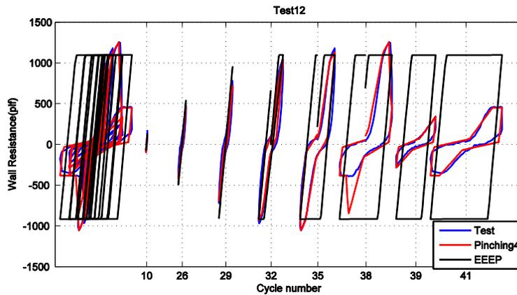
Figure 4: Pinching4 and EEEP model compared with Test 12 of Liu et al. (2012)
