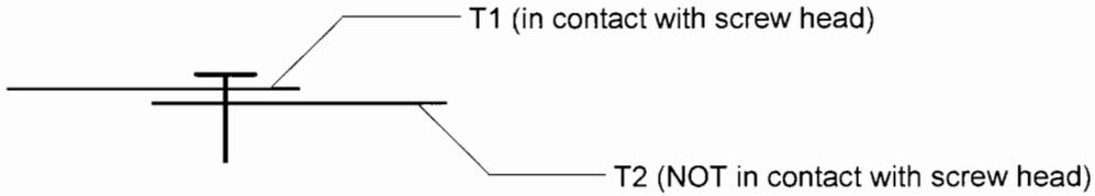
**Screw Connection Input Parameters**
