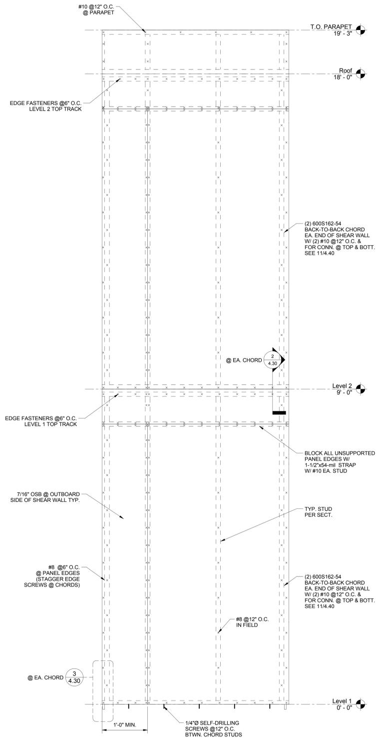
1 SHEAR WALL TYPE I ELEVATION
