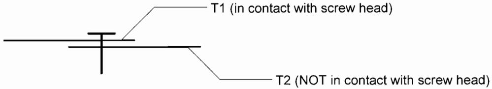
**Screw Connection Input Parameters**
