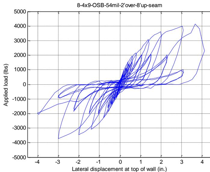
**Observed Failure Mode:** Fasteners at vertical seam (without additional stud ) pulled through OSB.
