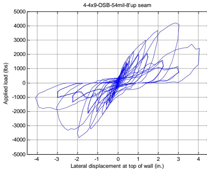
**Observed Failure Mode:** Fasteners in the seam location pulled through OSB.
