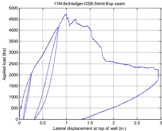
**Observed Failure Mode:** Failure at bottom OSB.(Bottom fastener spacing 12in. which is supposed to be 6in.).
