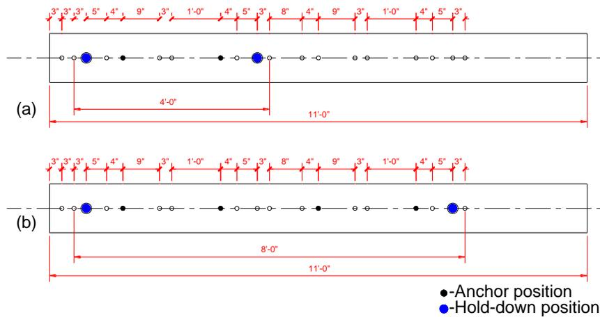
Figure 4 Anchor placements along frame base (top view) for (a) 4 ft and (b) 8 ft wide wall. (Large (blue) dots indicate hold down position and small black dots represent anchor position.)
