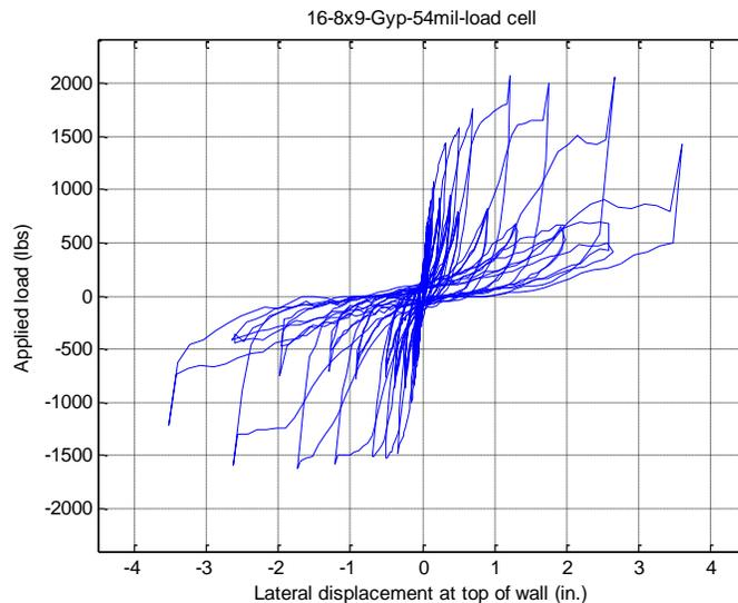
**Observed Failure Mode:** Screw holes enlarged; fasteners pulled through gypsum board. Gypsum board at chord studs has already separated.
