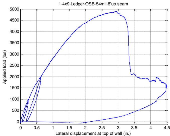
**Observed Failure Mode:** Failure occurred at bottom with fasteners tilted and pulled through the OSB.
