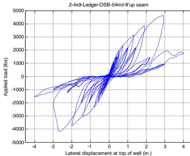
**Observed Failure Mode:** Failure occurred along the horizontal panel seam at 8' height with Fasteners tilted and then pulled through the OSB.
