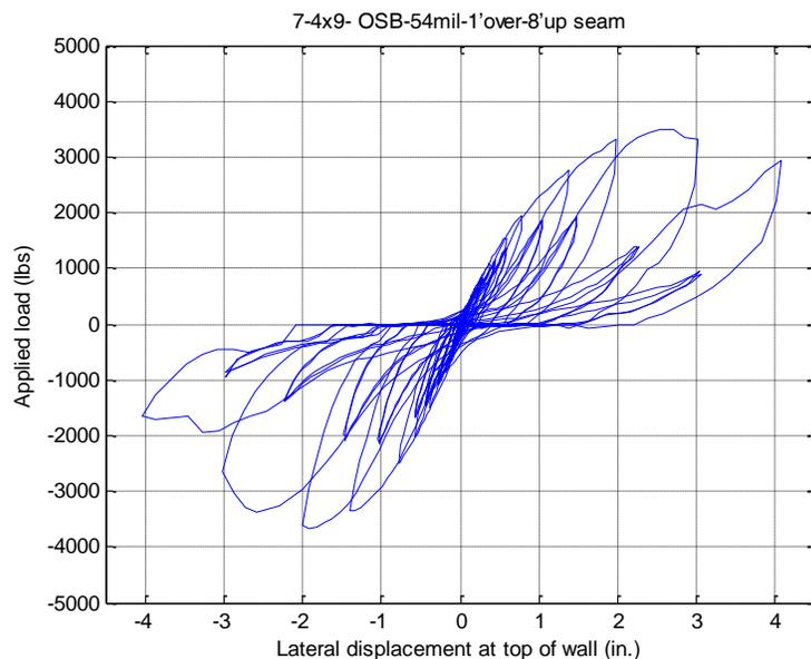
**Observed Failure Mode:** Failure occurred at vertical and horizontal seam, fasteners tilted and pulled through the OSB.
