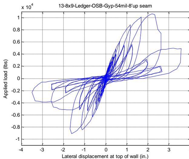
**Observed Failure Mode:** Failure occurred at OSB bottom and gypsum board. Fasteners at gypsum board enlarge holes, major of fasteners pull through board. South side gypsum board already separated from the frame. OSB side, bottom fasteners at bottom and chord stud up to 2' pulled through OSB.
