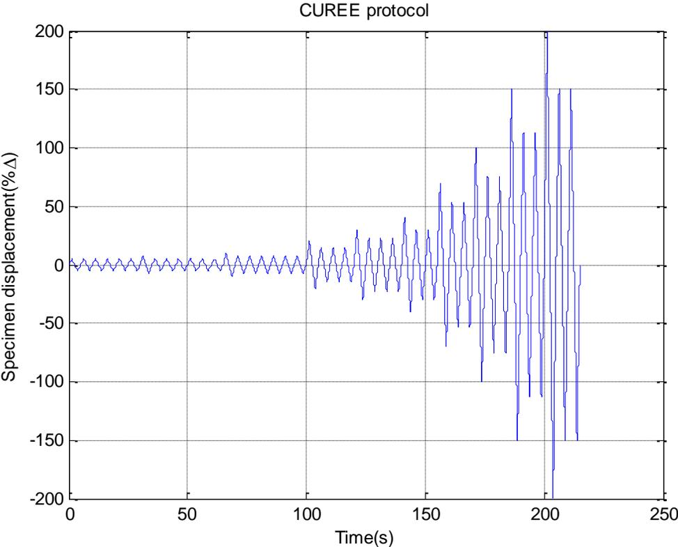
Figure 5 CUREE loading history as realized in a test
