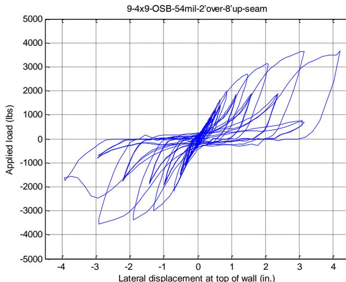
**Observed Failure Mode:** Fasteners at one side vertical seam pulled through OSB.
