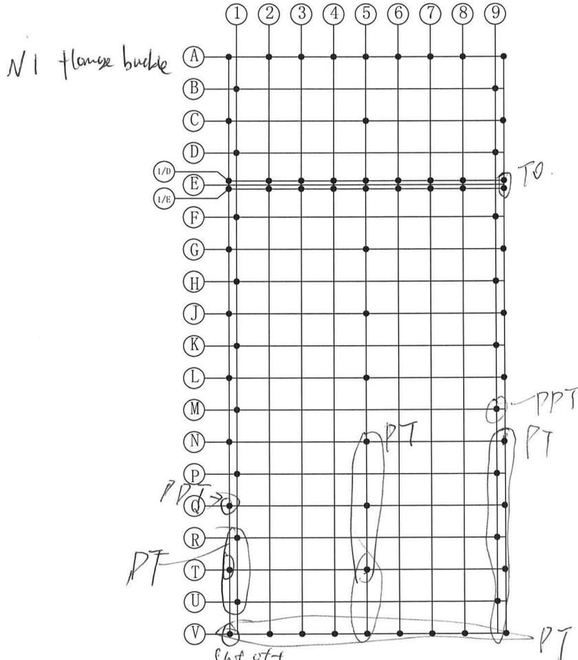
Failure mode: Pullout, withdrawal (PO); Fatigue Fracture Failure (FF); Pull through sheathing (PT);
