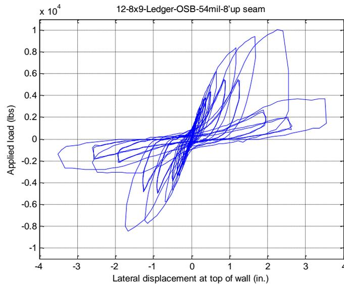
**Observed Failure Mode:** Fasteners at chord studs from bottom up to 2' up pulled through OSB.
