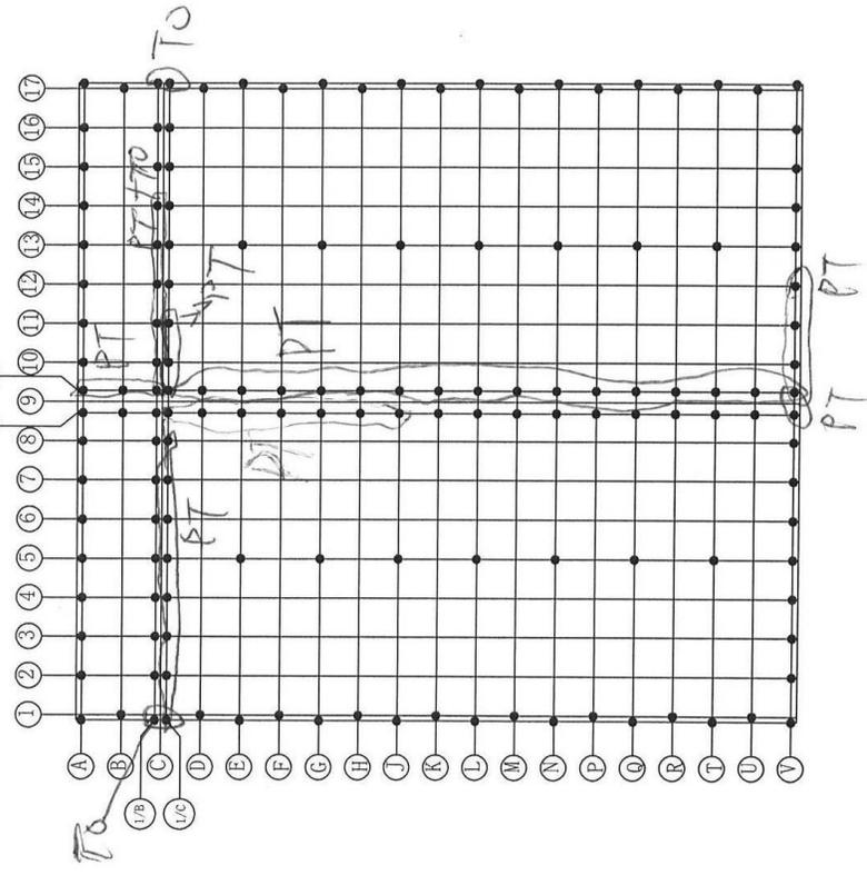
Failure mode: Pullout, withdrawal(PO); Fatigue Fracture Failure(FF); Pull through sheathing(PT);
