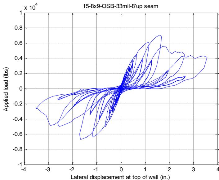
**Observed Failure Mode:** Failure occurred at vertical and horizontal seam with fastener tilted and pulled through OSB.
