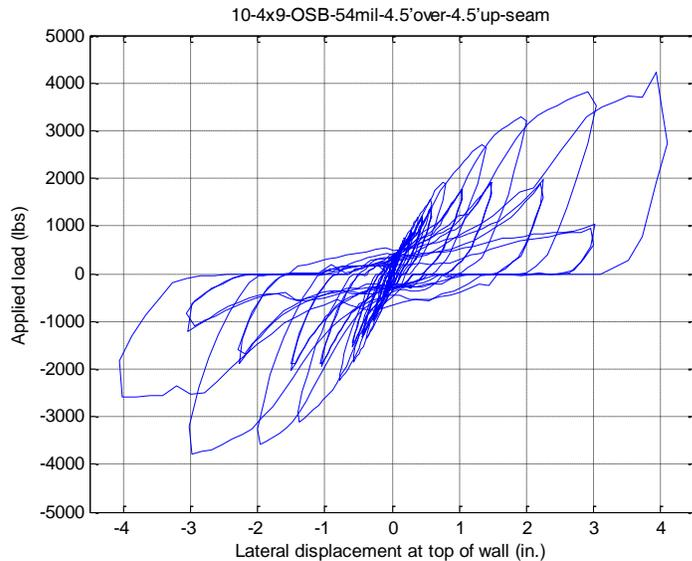
**Observed Failure Mode:** Fasteners at vertical seam location (south bottom part of OSB) pulled through OSB.
