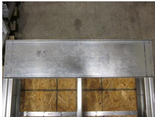
(a) Ledger attached to top of shear wall
