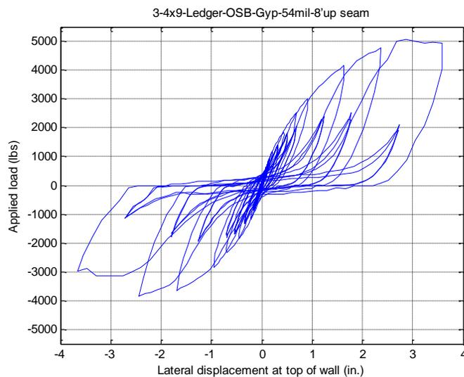
**Observed Failure Mode:** Fasteners on north chord stud all pulled through OSB, the screw hole was enlarged on the gypsum board.
