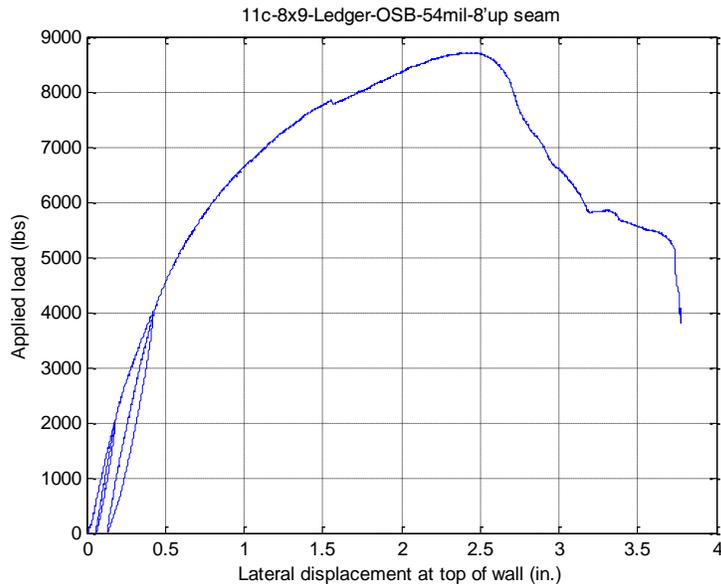
**Observed Failure Mode:** Failure occurred at vertical seam with wood bearing failure and fasteners pulled through OSB. .
