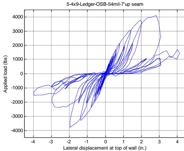
**Observed Failure Mode:** Failure occurred at the bottom of the OSB, fasteners tilted and then pulled through the OSB.
