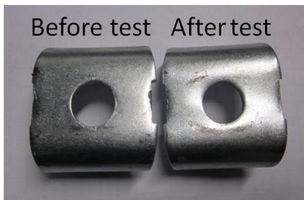
Figure 10 Deformation of hold-down (view from bottom, test 12 shown)
