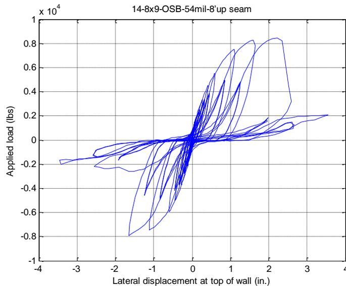
**Observed Failure Mode:** Failure occur at bottom fasteners pull through OSB, fasteners at chord studs up to 3' pull through and several wood bearing failures observed.
