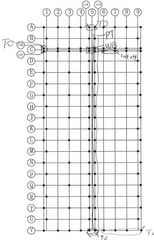
Failure mode: Pullout, withdrawal(PO); Fatigue Fracture Failure(FF); Pull through sheathing(PT);
