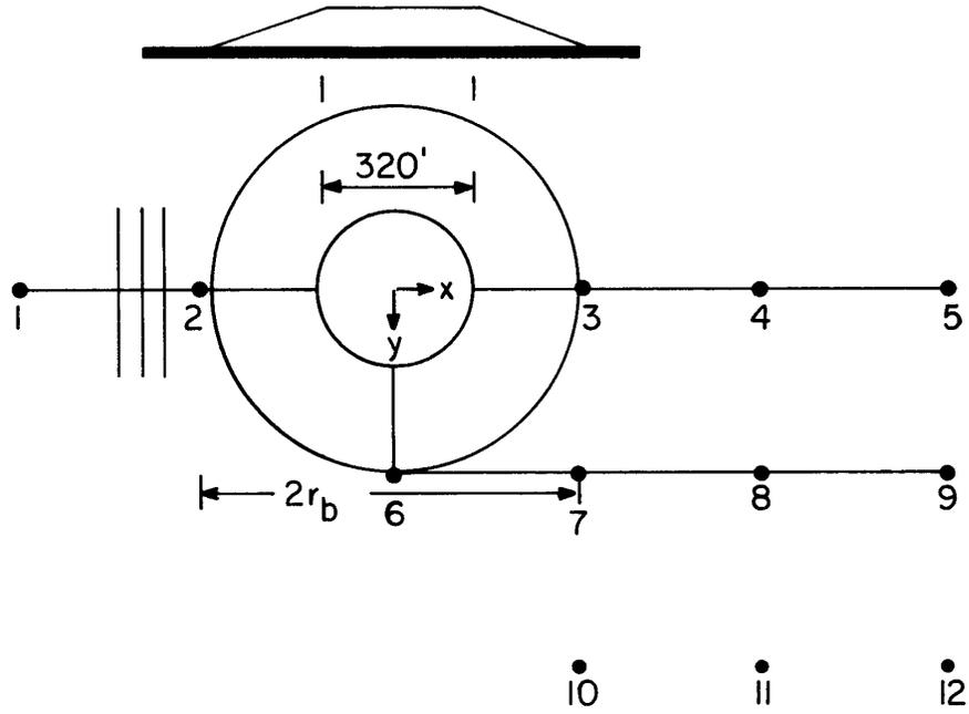
Figure 10: Locations for wave height measurements
