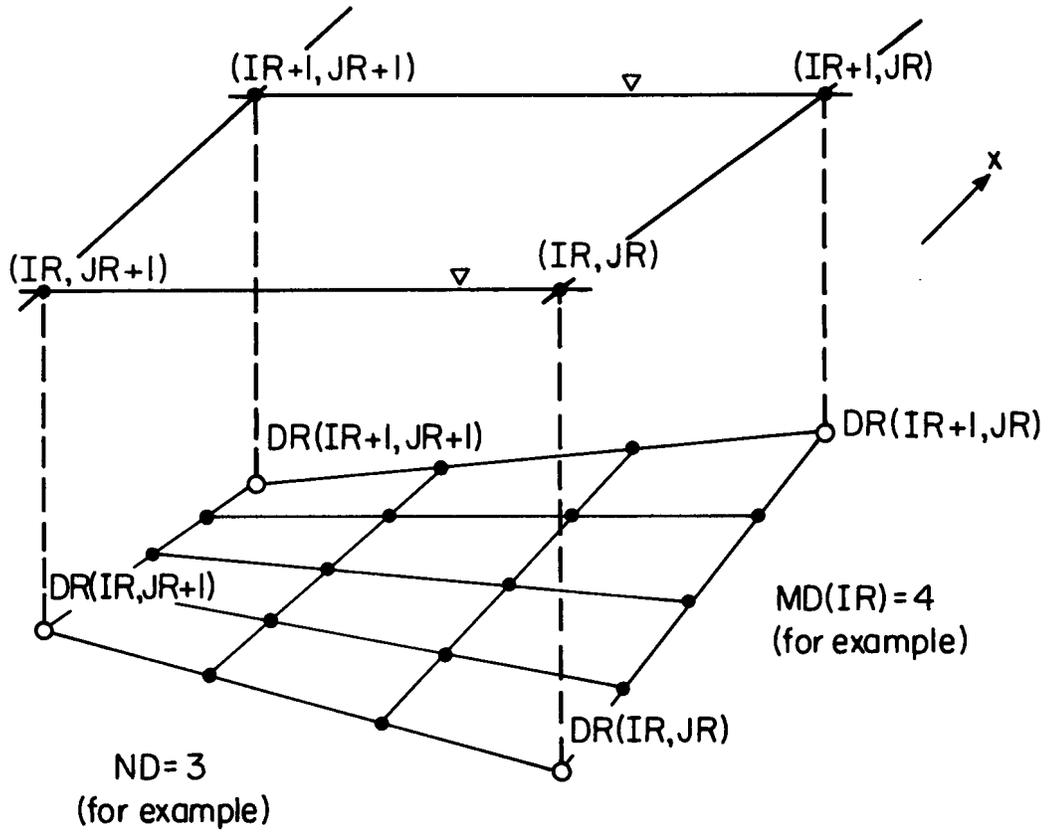
Figure 5: Interpolation of depth data
