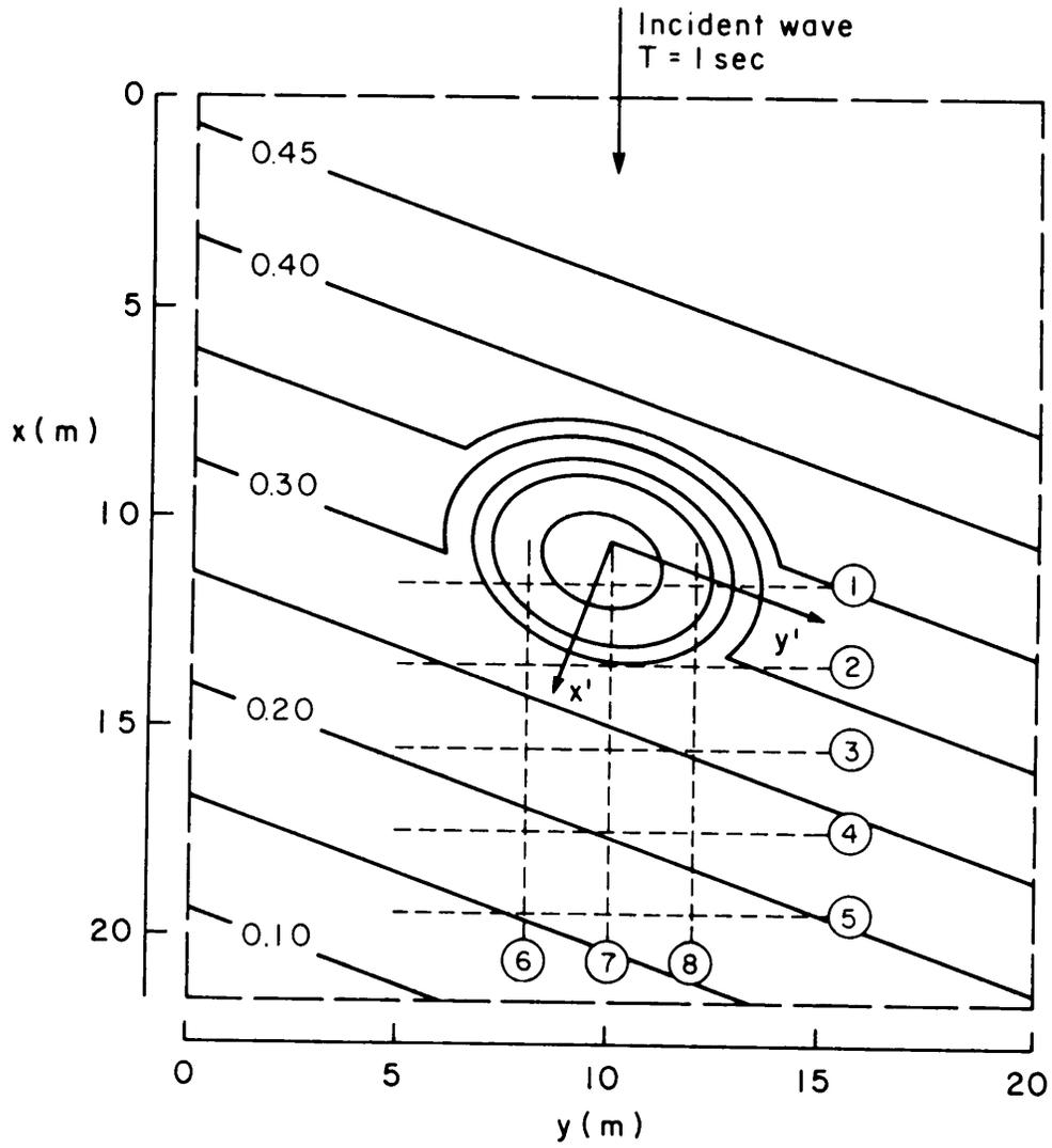
Figure 15: Bottom contours and computational domain for the experiment of Berkhoff et al (1982). Experimental data on transects 1-8.
