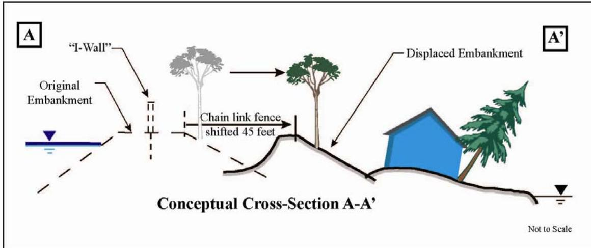
Figure 2.7: Schematic cross section at the 17<sup>th</sup> Street breach section.
